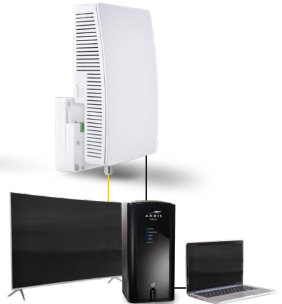
As demarcation point for Active Ethernet/ GPON/XGSPON ( Layer 2 "2 Box" approach )
